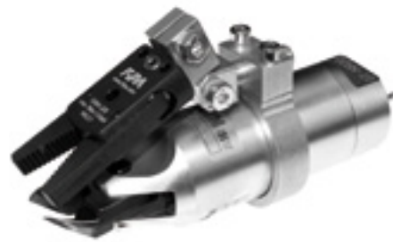
Gripping of sprue during cutting process
