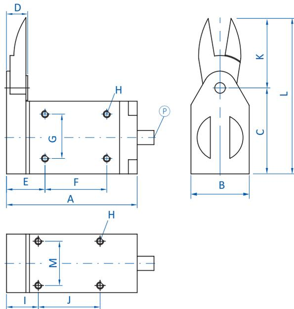
Ⓟ = Compressed air connection 4 mm x 2.5 mm
